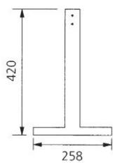
Standard console for fixed installation with central support
