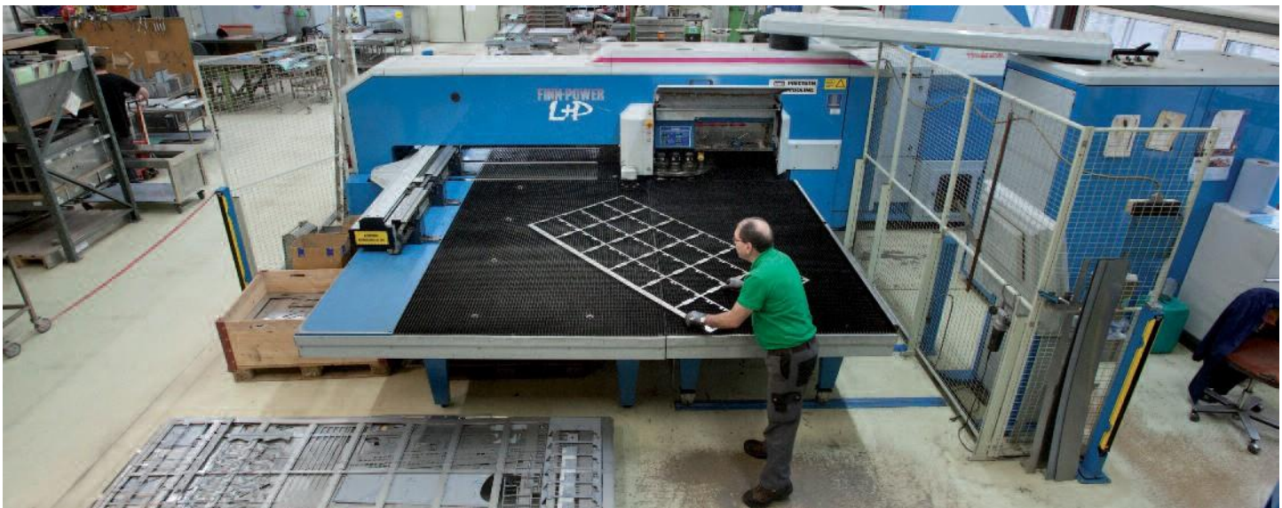
On the Finn Power laser punching machine, the individual parts are produced from large sheet metal plates.
